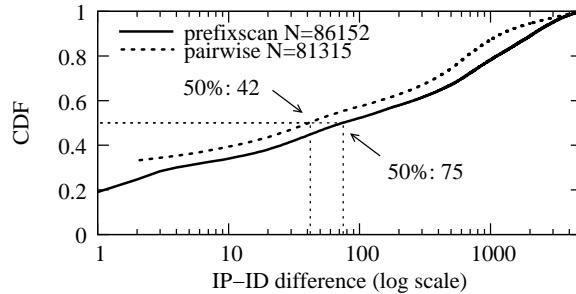
**Fig. 2.** IPID differences between inferred aliases A and A'. The smaller the difference, the more likely the alias inference is reliable. In our pairwise measurements, we rejected 4,837 initial pt2pt link inferences because either the IPIDs did not monotonically increase, or the counters increased too fast to reliably infer aliases. Of the 81K links remaining, 33% of the IPID values were strictly incremented between alias pairs.
