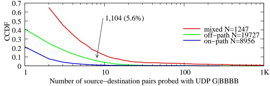
**Fig. 4.** CCDF of the number of source-destination pairs an interface was observed in a traceroute path, grouped by classifications made with UDP G|BBBB probes and the technique from [14]. 1,104 (5.6%) of interfaces were consistently inferred to be off-path using the technique from [14] that we infer to represent the in-bound interface of the router were traversed in at least eight source-destination pairs in our data.
