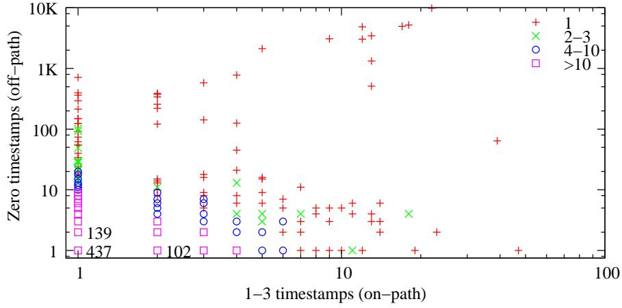
**Fig. 5.** Scatter plot of in-bound interfaces inferred to be on-path toward some destinations and off-path toward others (i.e. have mixed timestamp behavior). The symbol shape reflects the frequency of the on-path:off-path ratio in our data. Most interfaces are inferred to be on-path for just one source-destination pair using the technique from [14] despite being the in-bound interface of a pt2pt link.
