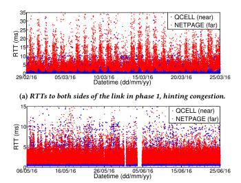
(b) RTTs to both sides of the link in phase 2: the diurnal pattern disappeared and congestion events were not seen until the end of the measurement period.
